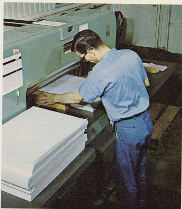
Del blocks a stack of paper in preparation for trimming with the Schimaneck cutter.
